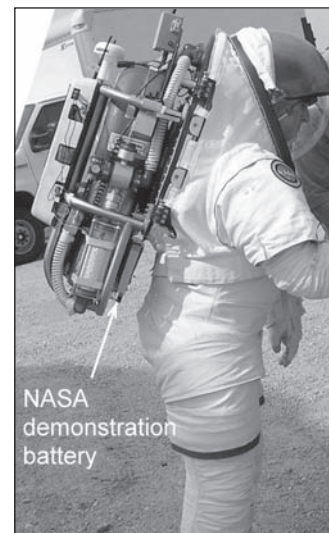
NASA Desert RATS battery installed on a spacesuit LAB.
