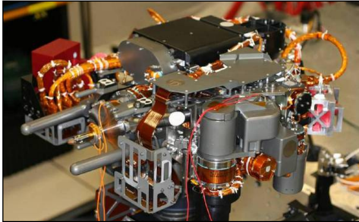
Figure 17. CHIMRA Installed on EM Turret
