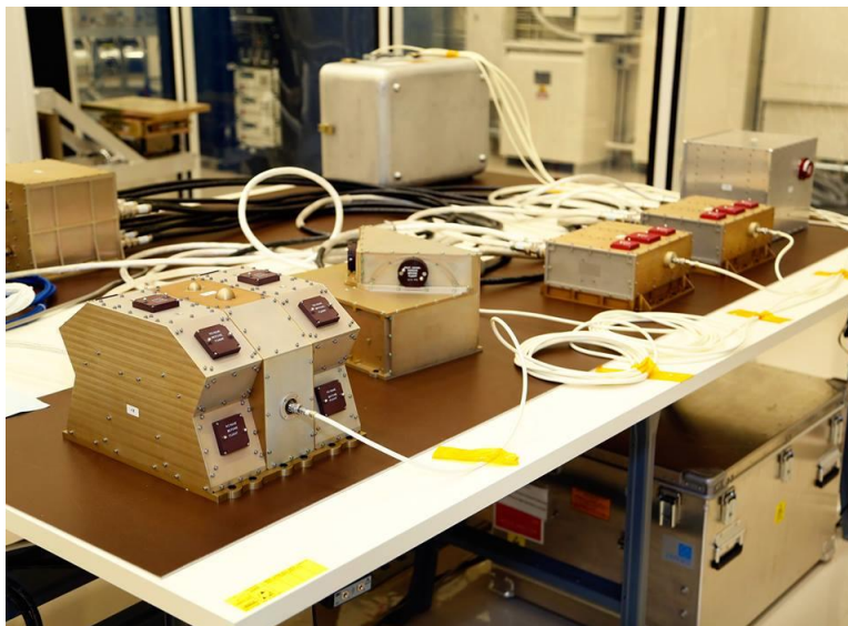
Figure 4: SEISS Instruments on the bench, from left to right: MPS-Hi, MPS-Lo, SGPS-1 & -2, and EHIS; DPU (back row, left) (Courtesy: Assurance Technology Corporation)
